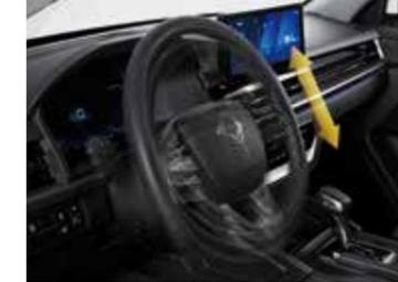
Tilt control of steering wheel angle
