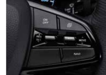
Steering wheel mounted cruise control switches
